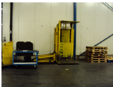
Recoup area with pallet converter
