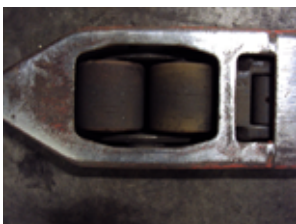
Tine of pallet jack with bogey suspension
