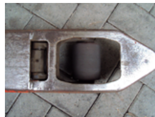
Tine of pallet jack without bogey suspension
