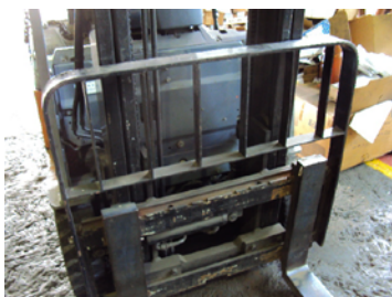
Pallet protector on forklift
